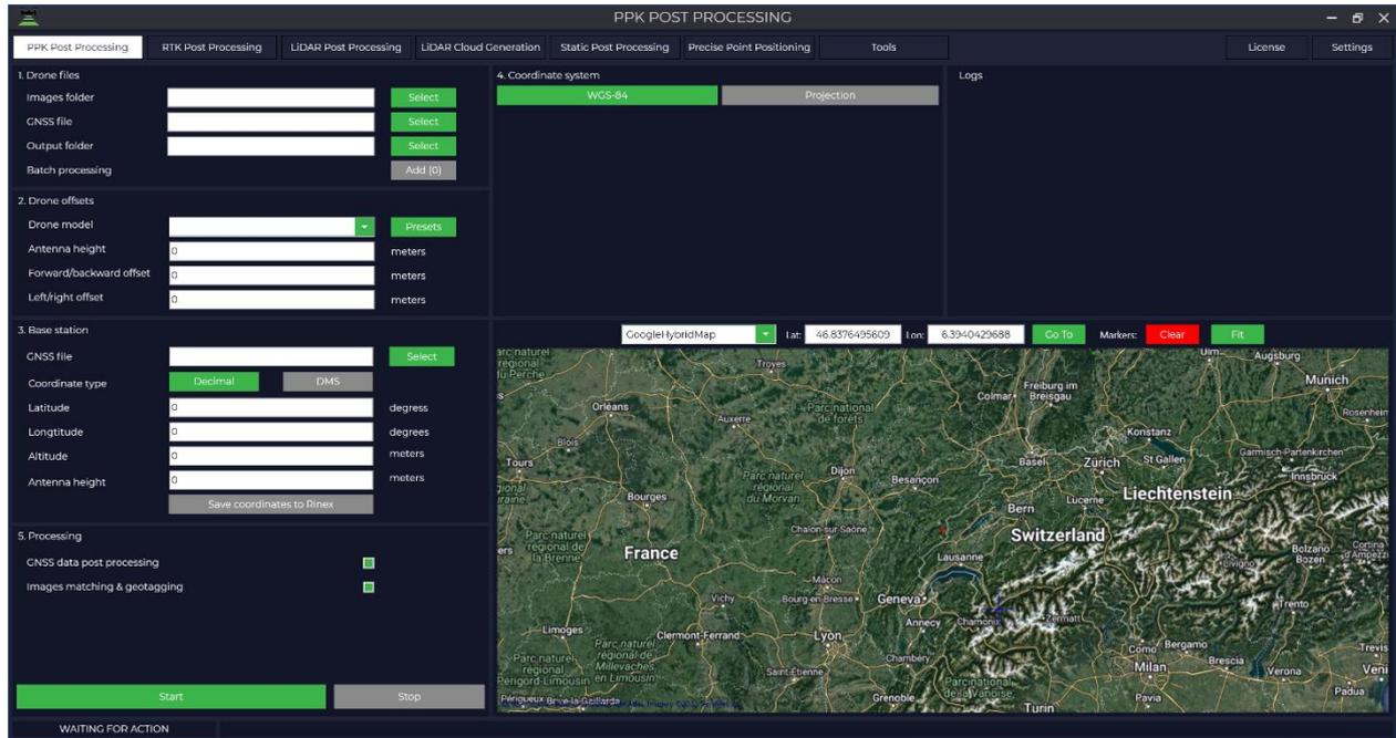
**TOPODRONE** Post Processing is a professional tool for automatic processing of the raw GNSS measurements at any coordinate system.
